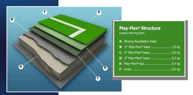
The flooring is durable, easy to lay, requires almost no maintenance and is resistant to abrasion and even the most aggressive weather conditions. Play-Flex is certified ITF - Class 1 (slow)
