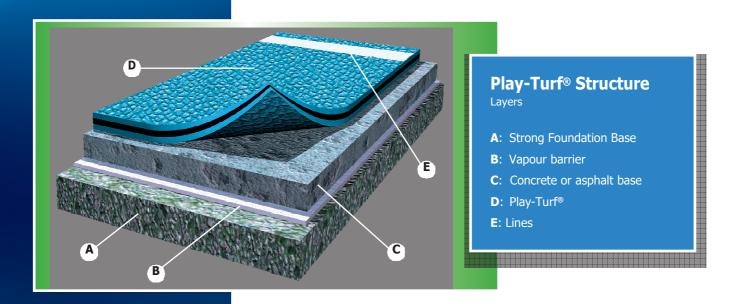
Specifically studied for covered Sports grounds and structures, Play-Turf® provides a calendared self-levelling polyvinyl chloride mantle. The ease and speed of the laying times make this an ideal flooring for all those sporting events which require a floor cover which can be quickly assembled and dissembled. In but 24 hours, it is possible to refurbish a sports field or decorate a gymnasium. Play-Turf® system is classified by ITF in Class 5 (fast).
